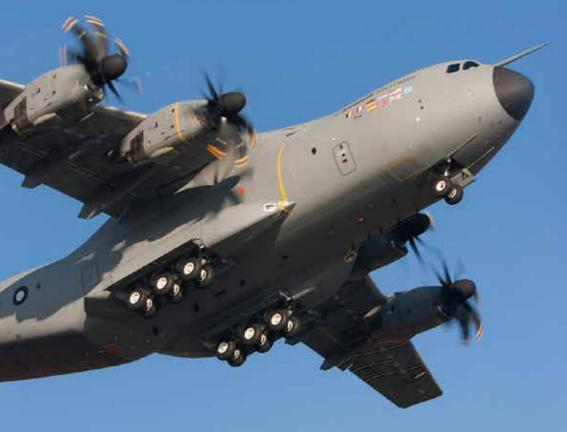
Successfully entered service in August 2013, the TP400-D6 is **the most powerful turboprop** engine in the West and has been developed to operate in the harshest environments. It is the first military engine to be fully civil certified from the outset by EASA in 2011.
